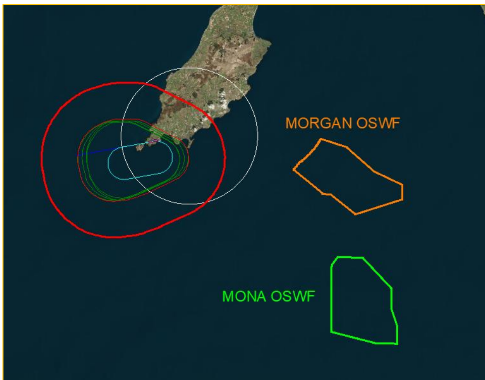
Figure 120 - Windfarms vs OFFSET ILS/DME RWY 08 Extended Holding
